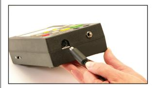
2. Attach the other end of the connection cable to the Tera Grand adapter:
