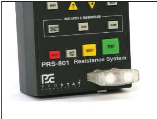
Figure 5: Low Resistance Range Calibration Shunt Installation. Note: The Shunt you received may look different than the ones in the photos.
