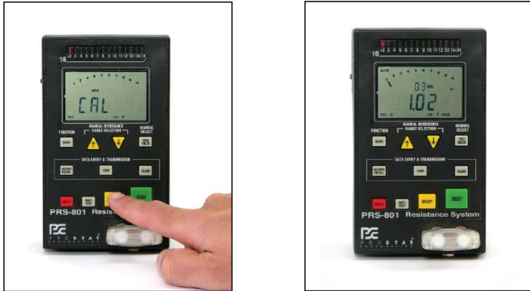
Figure 8: Complete Calibration Sequence by Pressing RESET. To confirm Calibration, Press TEST to measure the Calibration Shunt resistance. Shunt resistance should display 1.02 Ohms \pm 0.02 Ohms
