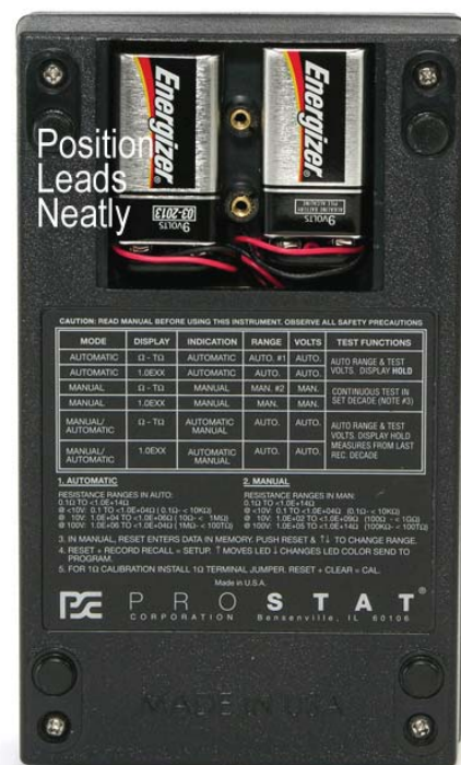
Figure 4: Install 2 each 9V Alkaline Batteries
