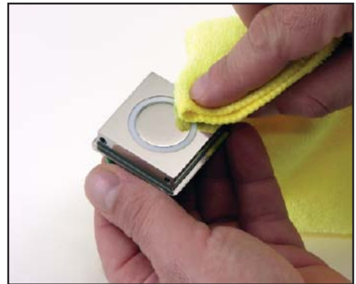
Figure 11: Cleaning Center Plate and Teflon Separator
