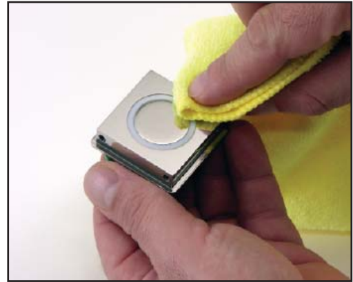
Figure 12: Cleaning the Power Plate with IPA and Micro Fiber Cloth
