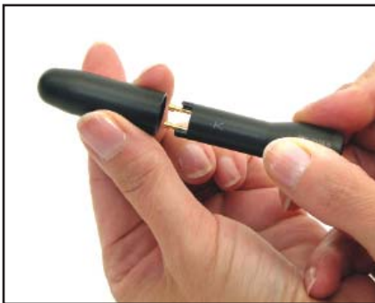
Figure 3: Remove Probe Cover
