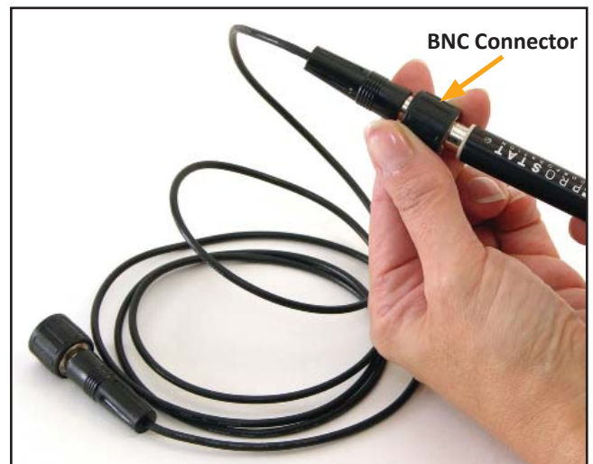
Figure 2: Connect shielded cable to host fixture BNC fitting
