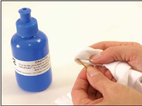
Figure 9: Cleaning the spring-loaded test
