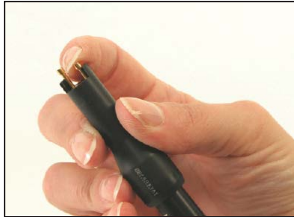
Figure 10: Insert Test Probe into its Socket and
