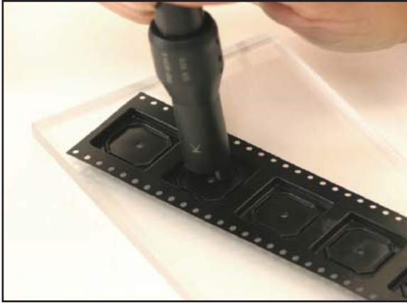
Figure 4: Measuring Carrier Tape
