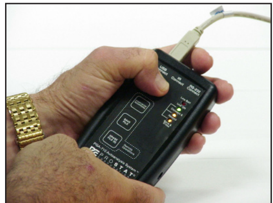
Figure 8: ON/OFF: Power up or place PGA-710 into "sleep mode".
