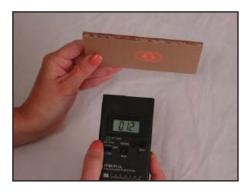
3. Position the front sensor of the PFM-711A Field Meter approximately one inch from the surface or object being measured. Move the instrument toward, or away from the surface until the RED Bulls Eye is focused on the test surface.
