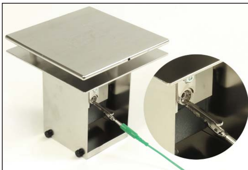
Figure 14: Grounding to the PFM-711A or PFM-711B
