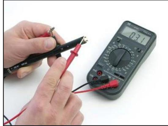
Figure 8: Measure pin continuity to the adapter banana to identify active measuring pin.
