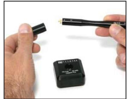
Figure 5: Remove Probe Cover
