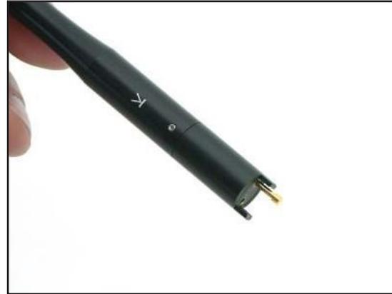
Figure 9: Removing the inactive pin helps identify point of actual measurement by the active pin.
