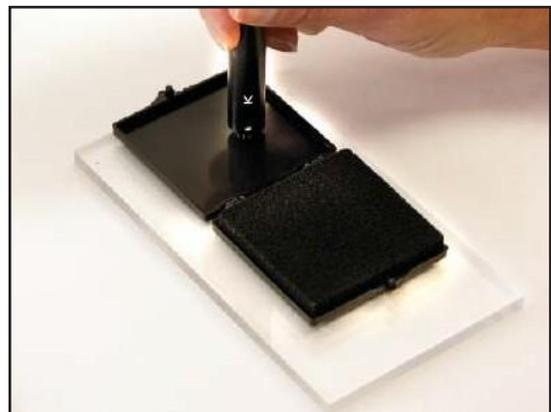
Figure 7: Measurement Illustrations Using the Prostat PRF-922B Fixture
