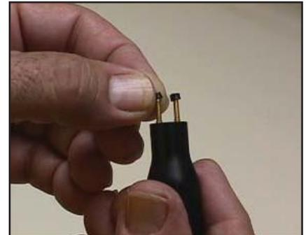
**Figure 9: Installing Conductive Rubber Electrode “Boots”**
