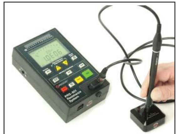
Figure 6: Insert PRF-922B Fixture into PRV-913B Two-Point Verifier and Measure Verifier Resistance
