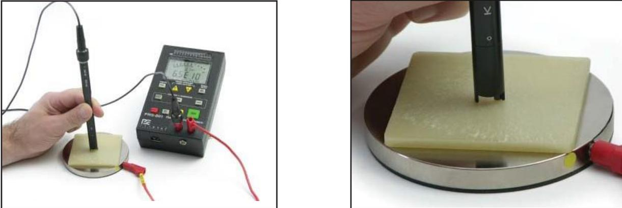
**Figure 10: Measurement setup for probe measurement of a material or device as described in ANSI/ESD STM11.13**
